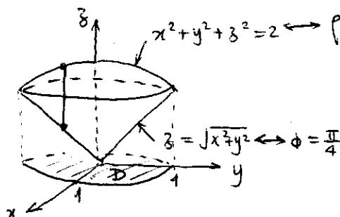
$$x^2 + y^2 + (x^2 + y^2) = 2 \Rightarrow \left\{ \begin{array}{l} x^2 + y^2 = 1 \\ z = \sqrt{x^2 + y^2} = 1 \end{array} \right.$$
